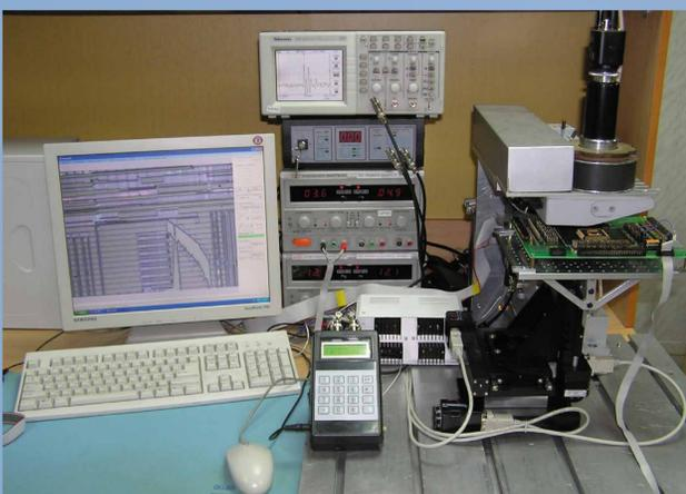
Portable design with nanosecond laser source, integrated into focusing unit (microscope)
