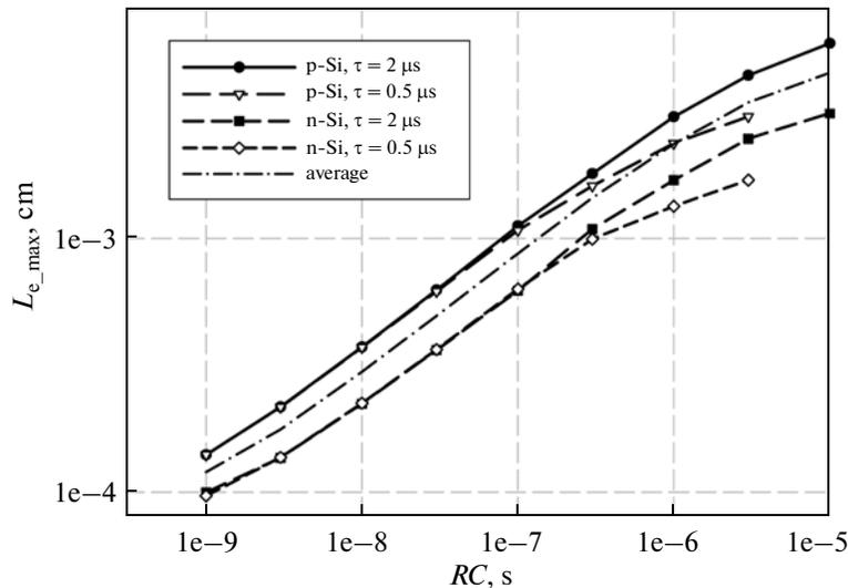
**Fig. 4.** Variations in the maximal collection length in *n*-type and *p*-type substrates against equivalent time constant  $RC$ .
