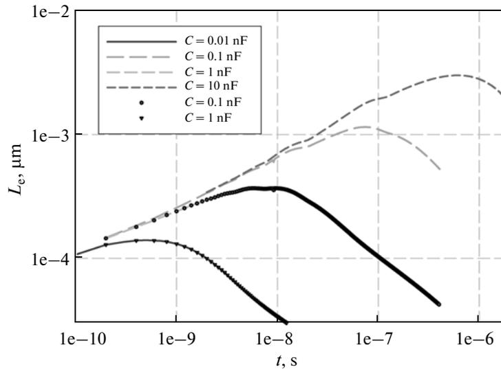
**Fig. 2.** Variation in the effective length in time for the semiconductor structure under the effect of the ionizing radiation pulse 70 ps wide and different values of  $C$ : curves  $R = 100 \Omega$ , symbols  $R = 10 \Omega$ .
