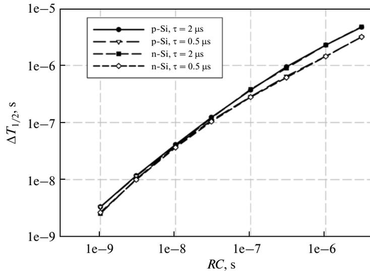
**Fig. 3.** Variations in the pulse width of the ionization reaction at a half-height in *n*-type and *p*-type substrates against the equivalent time constant  $RC$ .
