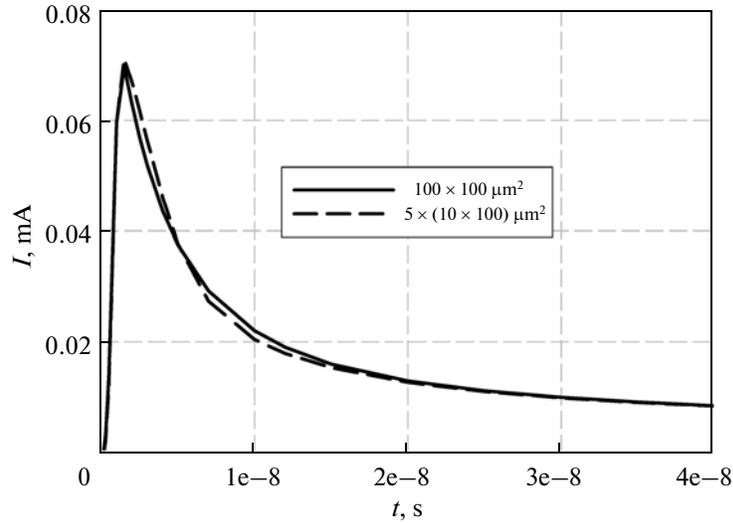
**Fig. 1.** Ionization current in a separate  $p-n$  junction and in the structure with five  $p-n$  junctions uniformly arranged on the crystal surface under the effect of the pulse of the ionizing radiation 70 ps wide.
